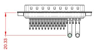
POWER/CO-AX CONTACT RATING:40A (CURRENT)(IF PRESENT)SIGNAL CONTACT CURRENT RATING:5A PER CONTACTSIGNAL CONTACT RESISTANCE: $10m\Omega$  MAX.INSULATOR RESISTANCE: $5000M\Omega$  min.DIELECTRICDIELECTRIC
