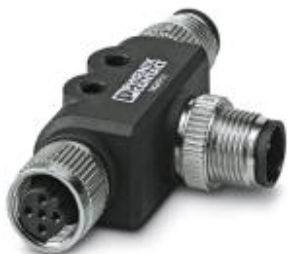
T distributor, PROFIBUS DP (12 Mbps), 5-position, shielded, Socket straight M12, B-coded, on Plug straight M12, B-coded and Plug straight M12, B-coded
