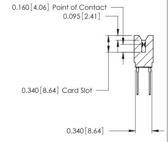
746 Series Ultra-Mate Card Edge Connector - Press Fit.
