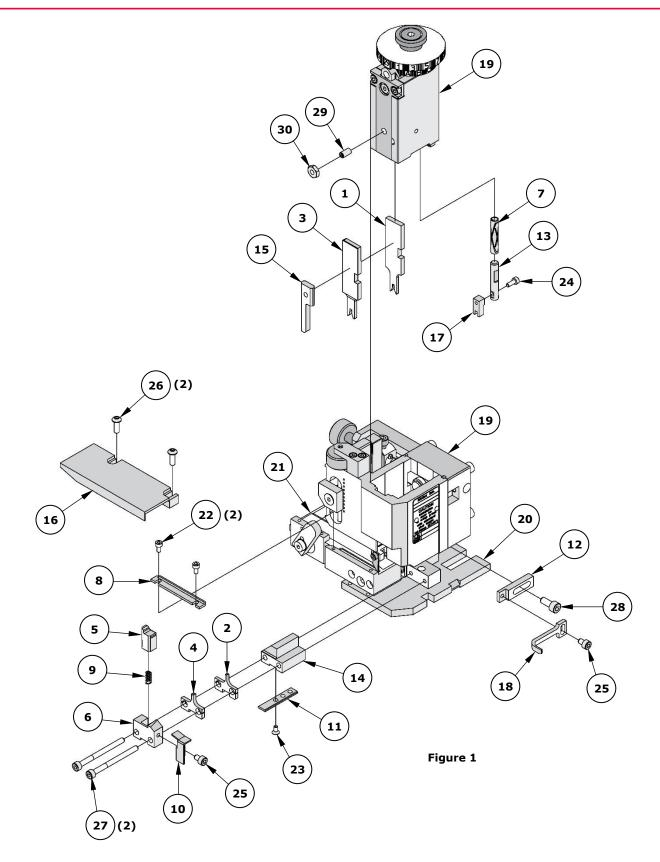
FineAdjust Applicator for Mega-Fit Wire-to-Wire Crimp Terminals
