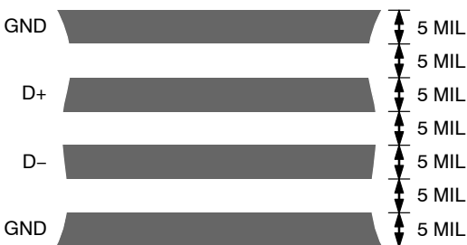
Figure 21. Typical Arrangement of Signal Tracks
