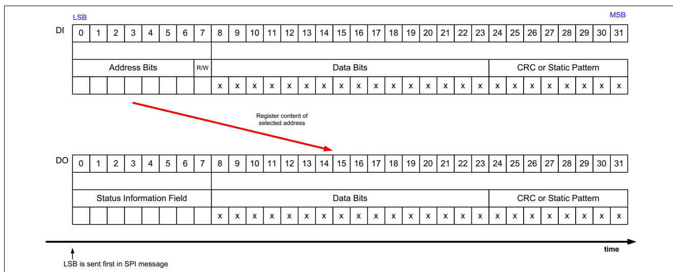
Figure 90 SPI Operation Mode
