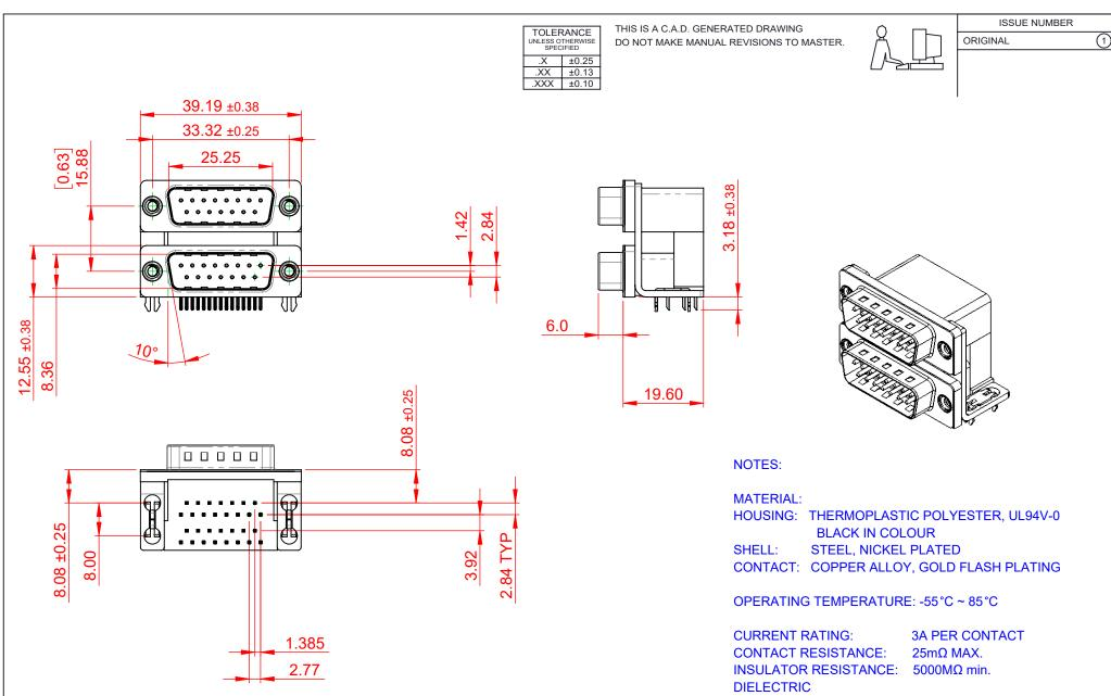
WITHSTANDING VOLTAGE: 1000V AC rms
