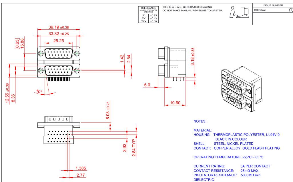
WITHSTANDING VOLTAGE: 1000V AC rms
