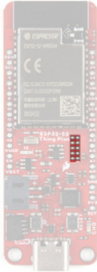
The JTAG pins on the ESP32-S2 Thing Plus. (Click to enlarge)
