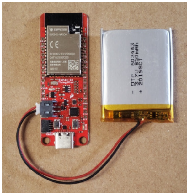
The ESP32-S2 Thing Plus with a battery connected. (Click to enlarge)
