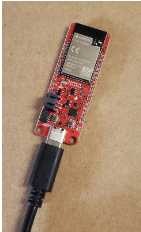
The ESP32-S2 Thing Plus with USB-C cable attached. (Click to enlarge)
