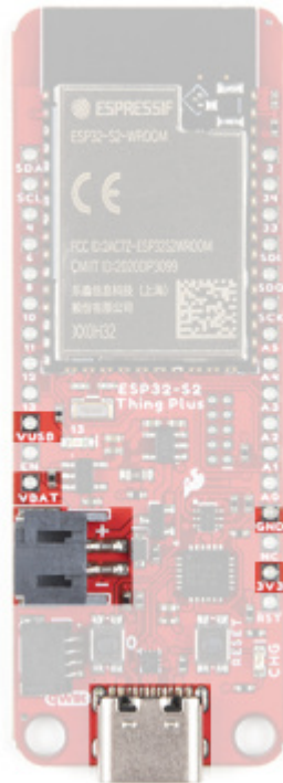
ESP32-S2 Thing Plus power connections. (Click to enlarge)
