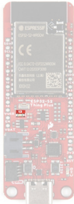
The status ( 13 ) LED indicator on the ESP32-S2 Thing Plus. (Click to enlarge)
