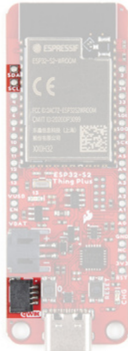
Qwiic connector and I 2 C pins on the ESP32-S2 Thing Plus. (Click to enlarge)
