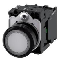
Illuminated pushbutton, 22 mm, round, plastic, clear, pushbutton, flat, momentary contact type, with holder, 1NO, LED module with integrated LED 24 V AC/DC, screw terminal, with laser labeling, upper case and lower case, always upper case at beginning of line
