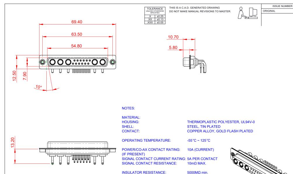
DIELECTRIC WITHSTANDING VOLTAGE: 1000V AC rms
