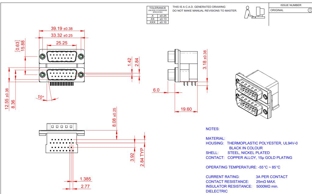
WITHSTANDING VOLTAGE: 1000V AC rms
