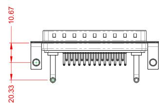
POWER/CO-AX CONTACT RATING:20A (CURRENT)(IF PRESENT)SIGNAL CONTACT CURRENT RATING:5A PER CONTACTSIGNAL CONTACT RESISTANCE:10mΩ MAX.INSULATOR RESISTANCE:5000MΩ min.DIELECTRIC5000MΩ min.
