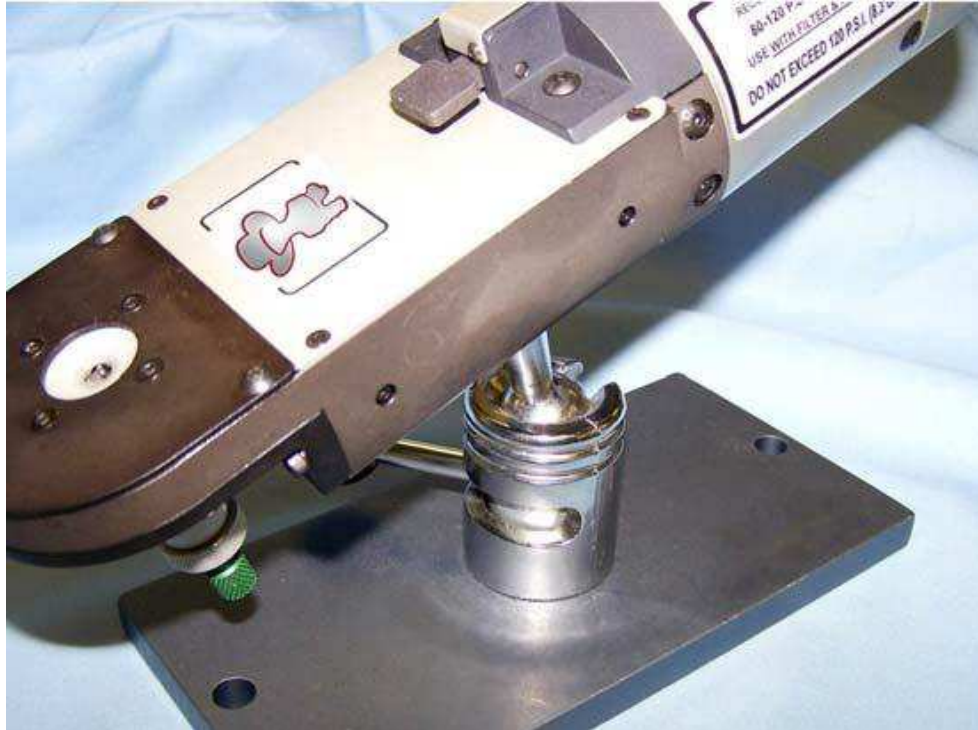
Figure 2: Ergonomics adjustment bench mount with locking arm to select tool angle
