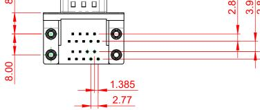
SHELL: STEEL, NICKEL PLATED CONTACT: COPPER ALLOY, GOLD FLASH PLATING (1)
