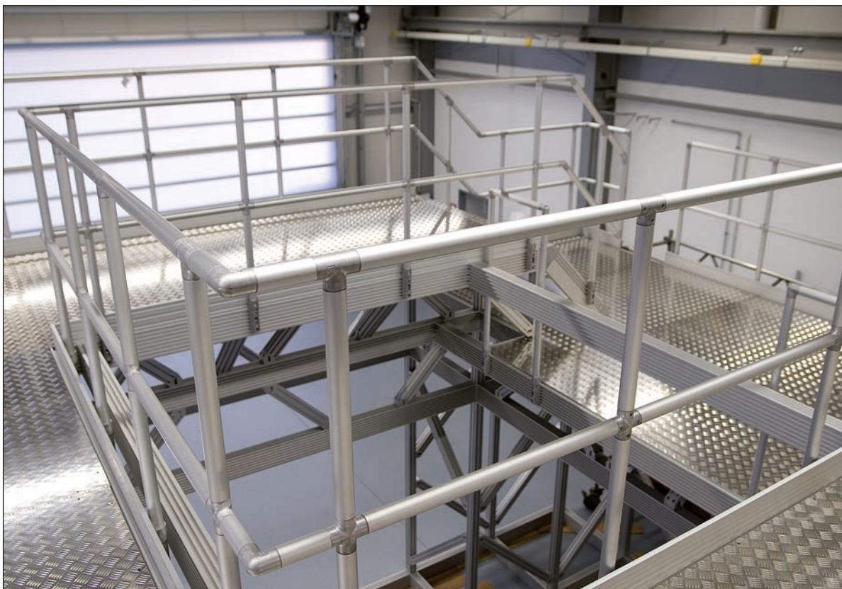
A circulating podium, in an assembly hall, with multiple access points.
