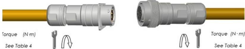
Step 13: Tighten metal nut
