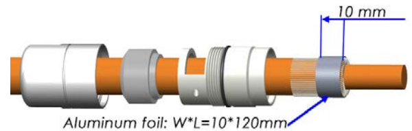
Step 4: Wrap foil over braided shielding
