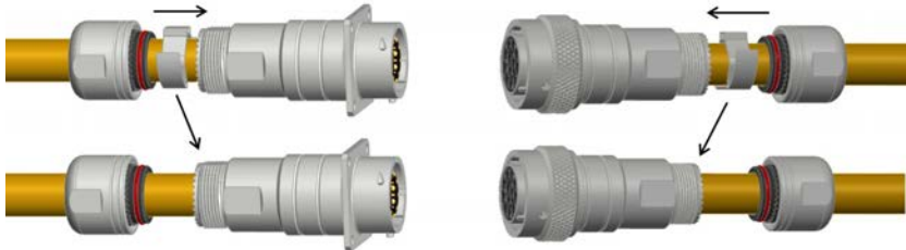
Step 11: Push shielding clip into backshell
