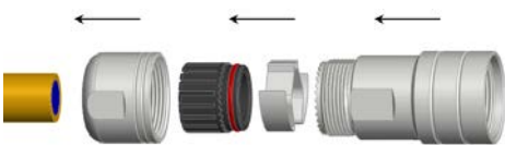
Step 1: Slide parts onto cable
