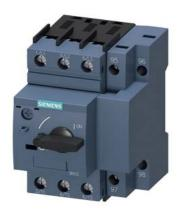
Circuit breaker size S00 for motor protection, CLASS 10 with overload relay function A-release 0.35...0.5 A N-release 6.5 A screw terminal Standard switching capacity
