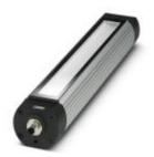
LED machine light, 24 V DC, emission angle 75 °/95 °, color temperature 5000 K, length 370 mm, diameter 70 mm, M12 connector, Light housing: Anodized aluminum, Pane: Single-pane safety glass (ESG, thermally toughened float glass), pivoting, resistant to coolants and lubricants
