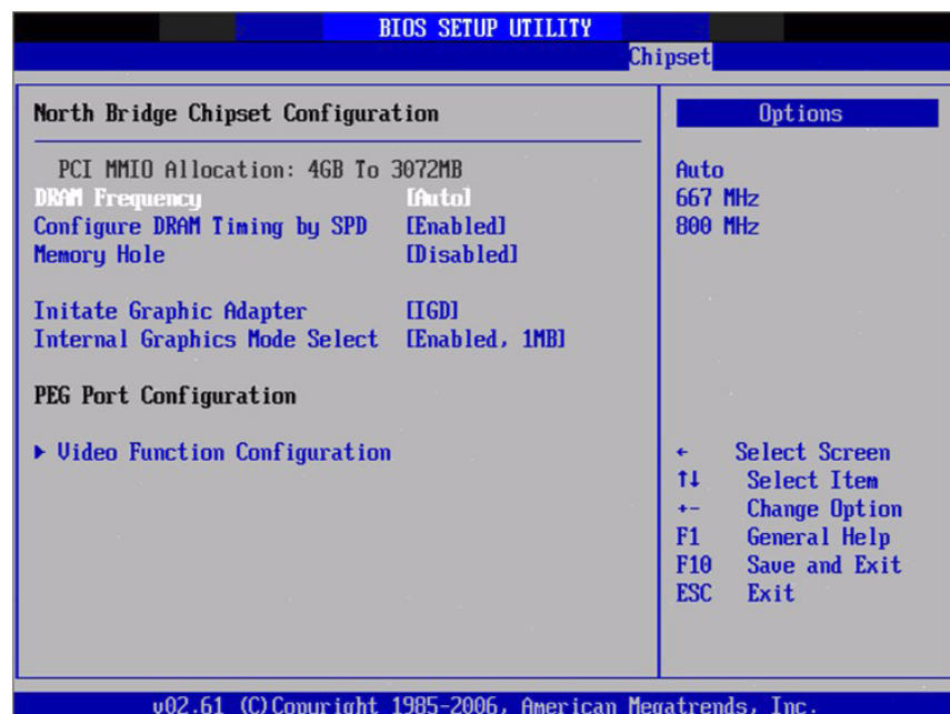
Figure 3.23 North Bridge Configuration
