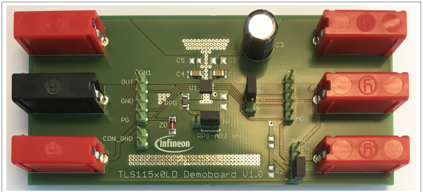
Figure 3 OPTIREG™ linear voltage regulator TLS115x0LD demoboard
