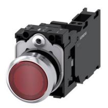
Illuminated pushbutton, 22 mm, round, Metal, shiny, red, pushbutton, flat, momentary contact type, with holder, 1 NO+1 NC, LED module with integrated LED 230 V AC, spring-type terminal, with laser labeling, symbol number according to, ISO 7000 or IEC 60417
