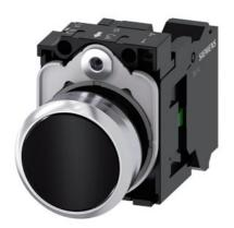
Pushbutton, 22 mm, round, metal, shiny, black, pushbutton, flat, momentary contact type, 1 NO, spring-type terminal, with laser labeling, upper case and lower case, always upper case at the beginning of the word
