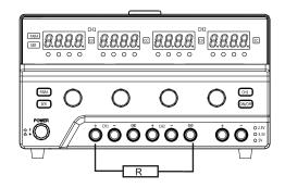
2. The Parallel Operation: Press and hold the button PARA for 1 seconds to be in the parallel mode. When the PARA indicator on the display lights on, it means the power supply is in the parallel mode now. At this mode, CH2 is the master operation while CH1 is the slave operation, when the CH1 operation is shielded. At this time, press the button ON/OFF and then the output can be turned on or off. And the output connection is as shown in the figure:
