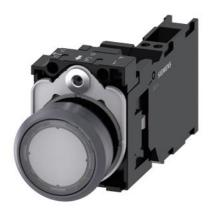
Illuminated pushbutton, 22 mm, round, plastic with metal front ring, clear, pushbutton, flat, momentary contact type, with holder, 1 NO+1 NC, LED module with integrated LED 24 V AC/DC, spring-type terminal, with laser labeling, inscription or symbol Customer-specific selection with SIRIUS ACT configurator (CIN)
