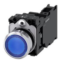
Illuminated pushbutton, 22 mm, round, metal, shiny, blue, pushbutton, flat, momentary contact type, with holder, 1 NO+1 NC, LED module with integrated LED 24 V AC/DC, spring-type terminal, with laser labeling, inscription or symbol Customer-specific selection with SIRIUS ACT configurator (CIN)
