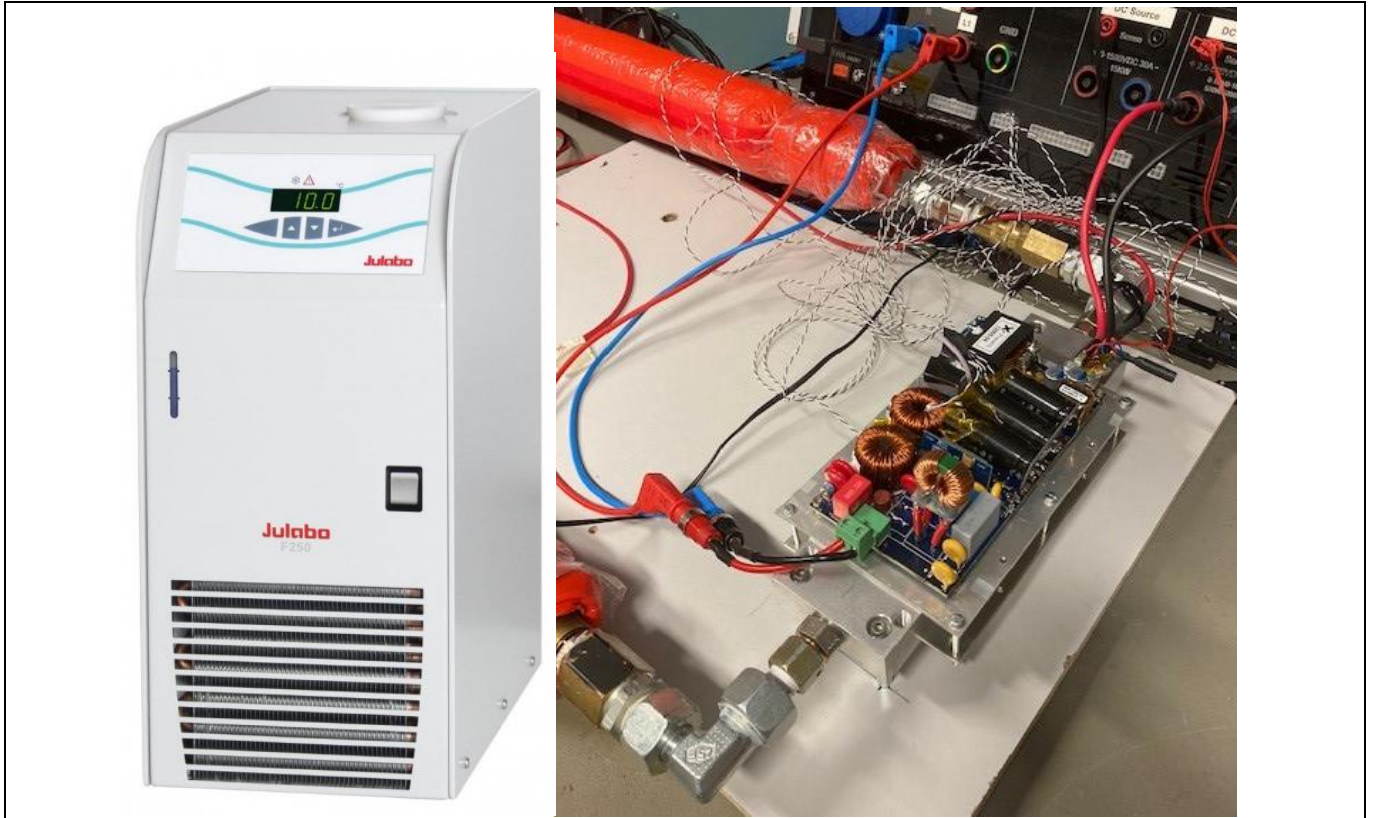
Figure 36 Thermal characterization test bench based on water cooling
