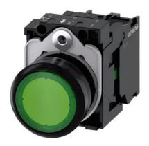
Illuminated pushbutton, 22 mm, round, plastic, green, pushbutton, flat, momentary contact type, with holder, 1NO, LED module with integrated LED 110 V AC, screw terminal, with laser labeling, upper case and lower case, Always upper case at the beginning of the word
