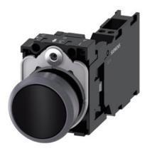
Pushbutton, 22 mm, round, plastic with metal front ring, black, pushbutton, flat, momentary contact type, with holder, 1 NO+1 NC, spring-type terminal, with laser labeling, symbol number according to, ISO 7000 or IEC 60417
