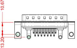
30A (CURRENT) **POWER/CO-AX CONTACT RATING:** (IF PRESENT) SIGNAL CONTACT CURRENT RATING: 5A PER CONTACT SIGNAL CONTACT RESISTANCE:  $10m\Omega$  MAX.
