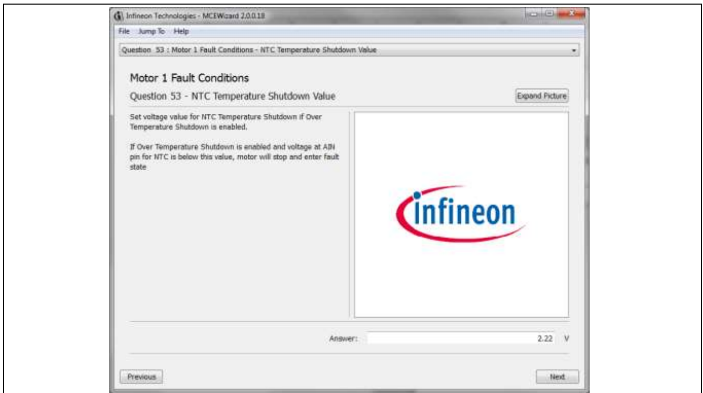
Figure 18 External temperature sense input configuration in MCEWizard
