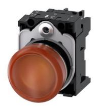
Indicator lights, 22 mm, round, metal, shiny, amber, lens, smooth, with holder, LED module with integrated LED 24 V AC/DC, screw terminal, Z=20-unit packaging
