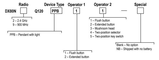
The Q120PPB has two operator inputs and one four-color LED indicator light output.
