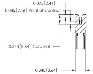
ACAD REFERENCE NO. 746 Series Ultra-Mate Card Edge Connector - Press Fit DRAWN: J.LEE Part Number: 746-042-540-606 CHECKED: **EDAC INC** SCALE: THESE DRAWINGS AND SPECIFICATIONS ARE THE PROPERTY OF EDAC INC.,AND TORONTO, ONTARIO SHALL NOT BE REPRODUCED, OR COPIED DRAWING NUMBER CANADA OR USED AS THE BASIS FOR THE 746-ENG MASTER MANUFACTURE OR SALE OF APPARATUS YOUR CONNECTION TO QUALITY & SERVICE WITHOUT WRITTEN PERMISSION.
