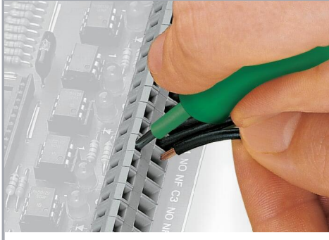
Inserting a conductor via 3.5 mm screwdriver.
