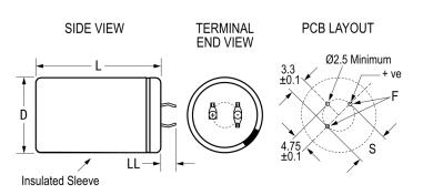
General Information Series ALC80 Dielectric Aluminum Electrolytic Description Snap-In, Aluminum Electrolytic RoHS Lead 3 Pin Short AEC-Q200 No Halogen Free Yes Component Weight 50 g Notes Dimensions D And L Include Sleeving. Shelf Life 156 Weeks
