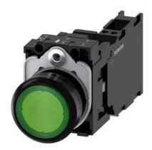
Illuminated pushbutton, 22 mm, round, plastic, green, pushbutton, flat, momentary contact type, with holder, 1 NO+1 NC, LED module with integrated LED 24 V AC/DC, spring-type terminal, with laser labeling, inscription or symbol Customer-specific selection with SIRIUS ACT configurator (CIN)
