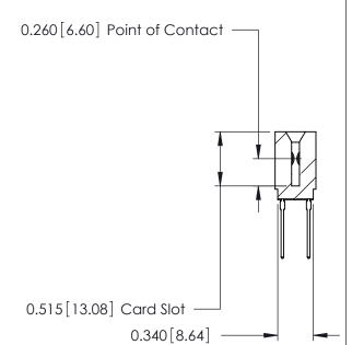
ACAD REFERENCE NO. 746-ENG MASTER 746 Series Ultra-Mate Card Edge Connector - Press Fit DRAWN: DATE: AUG 20/09 J.LEE Part Number: 746-036-540-201 CHECKED: DATE: **EDAC INC** SCALE: SHEET 1 OF 1 THESE DRAWINGS AND SPECIFICATIONS ARE THE PROPERTY OF EDAC INC.,AND TORONTO, ONTARIO SHALL NOT BE REPRODUCED, OR COPIED DRAWING NUMBER CANADA OR USED AS THE BASIS FOR THE 746-ENG MASTER MANUFACTURE OR SALE OF APPARATUS YOUR CONNECTION TO QUALITY & SERVICE WITHOUT WRITTEN PERMISSION.
