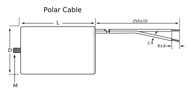
General Information Series C28 Dielectric Film/Foil Polypropylene Style Plastic Case and Cover, Ultra Sonically Welded Description Ultra Sonically Welded Seal, Safety Class S3, UL\_94 V0 Disk **Features** RoHS Yes Termination Tin Copper Lead Cables UL, VDE, UL (Construction Only), UL\_94 VO Disk Qualifications AEC-Q200 Component 38.87 g Weight
