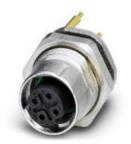
Bus system flush-type socket, Ethernet, 4-pos., M12 SPEEDCON, shielded, D-coded, rear/screw mounting with Pg9 thread, with straight solder connection, design with 12 mm long solder pins
