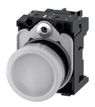
Indicator light, 22 mm, round, plastic, white, lens, smooth, with holder, LED module, with integrated LED 24 V AC/DC, screw terminal, with laser labeling, upper case and lower case, always upper case at beginning of line
