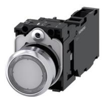
Illuminated pushbutton, 22 mm, round, Metal, shiny, clear, pushbutton, flat, momentary contact type, with holder, 1 NO+1 NC, LED module with integrated LED 230 V AC, screw terminal, with laser labeling, inscription or symbol Customer-specific selection with SIRIUS ACT configurator (CIN)
