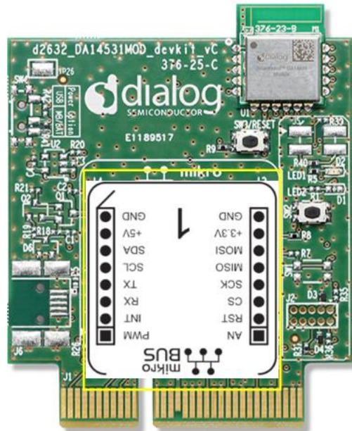
Figure 18: Example of mounting MikroBUS™ module
