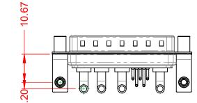
30A (CURRENT) POWER/CO-AX CONTACT RATING: (IF PRESENT) SIGNAL CONTACT CURRENT RATING: 5A PER CONTACT SIGNAL CONTACT RESISTANCE:  $10m\Omega$  MAX. **INSULATOR RESISTANCE:**
