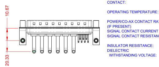
20A (CURRENT) POWER/CO-AX CONTACT RATING: (IF PRESENT) SIGNAL CONTACT CURRENT RATING: 5A PER CONTACT SIGNAL CONTACT RESISTANCE:  $10m\Omega$  MAX. **INSULATOR RESISTANCE:** 5000MΩ min. DIELECTRIC
