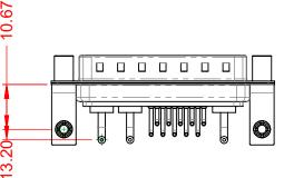
**OPERATING TEMPERATURE:** -55°C ~ 125°C 10A (CURRENT) POWER/CO-AX CONTACT RATING: (IF PRESENT) SIGNAL CONTACT CURRENT RATING: 5A PER CONTACT SIGNAL CONTACT RESISTANCE:  $10m\Omega$  MAX. INSULATOR RESISTANCE:
