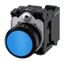
Pushbutton, 22 mm, round, plastic, blue, pushbutton, flat, momentary contact type, with holder 1 NO, spring-type terminal, with laser labeling, inscription or symbol Customer-specific selection with SIRIUS ACT configurator (CIN)
