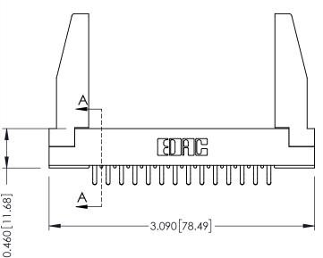
0.295[7.49] Card Slot SECTION 0.090[2.29] Point of Contact
