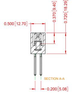
ACAD REFERENCE NO .: 317 Assembly 317 SERIES CARD EDGE CONNECTOR C.B DATE: February 5, 2020 DRAWN: CHECKED: DATE: THESE DRAWINGS AND SPECIFICATIONS OF SCALE: 1:1 SHEET 1 1 AC INC ARE THE PROPERTY OF EDAC INC..AND O, ONTARIO SHALL NOT BE REPRODUCED, OR COPIED 317-046-542-803 DRAWING NUMBER: ISSUE OR USED AS THE BASIS FOR THE NADA MANUFACTURE OR SALE OF APPARATUS 1 & SERVICE PART NUMBER: 317-046-542-803 WITHOUT WRITTEN PERMISSION.
