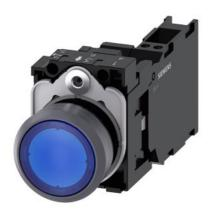
Illuminated pushbutton, 22 mm, round, plastic with metal front ring, blue, pushbutton, flat, momentary contact type, with holder, 1 NO+1 NC, LED module with integrated LED 24 V AC/DC, spring-type terminal, with laser labeling, lower case
